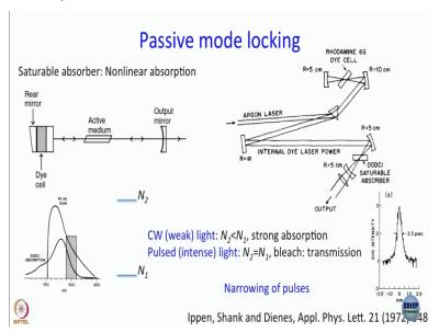
We will continue our discussion of mode locking and then go on to something called cavity dumping. This is where we have got until the last module, which we have discussed active mode locking using a mode locker by applying sound frequency using Debye Sears effects within the Raman Nath regime. And then we moved on to talk about passive mode locking, where what is used is saturable absorbers, so, and we have finished our discussion saying saturable absorber can not only produce pulses.
