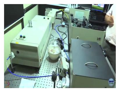
Alright this is the optical table on which our femtosecond optical gating experiment is done. This here is a femtosecond laser. In our case, it is a tsunami laser from new port it is quite old. The other laser that we have not shown you yet I think is much compact. But what tsunami does is that it provides 800 nanometer light with 100 femtosecond pulses at 80 megahertz repetition rate. So that light you can hardly see it comes here hits this mirror comes here goes to this optical unit.
