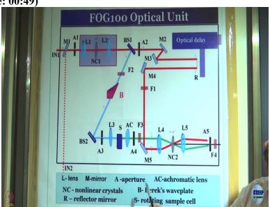
So you might remember that this is the layout of our optical unit for the fog spectrometer. The spectrometer we use in our lab has the name fog 100. It is from a company called CDP Corporation, which is based in Russia. So, just to remind you, what we have here is that we have red light, nominal, 800 nanometer, but in our case tunable from 690 nanometer all the way to 950 nanometer from a femtosecond pulse titanium Sapphire laser.
