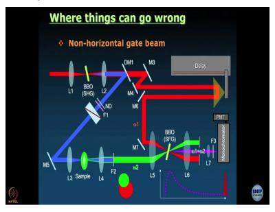
First mistake that can come and this is something that one needs to be very worried about is if the gate beam is not horizontal. Let us go back to the schematic. Remember, this decay that you are generating this map of the fluorescence decay is actually raw values of intensity. It is not a relative
