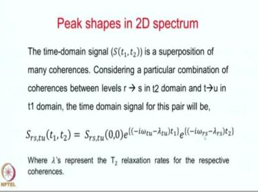
Considering a particular combination of coherences between levels r and s. Now r and s is taken in  $t_2$  domain and t to u in the  $t_1$  domain. The time domain signal for this pair will be  $S_{rs,tu}(t_1,t_2)$ and we have here, well in fact tu is  $\omega_{tu}$  is taken as in the  $t_1$  dimension and  $\omega_{rs}$  is taken as  $t_2$ dimension. Complex signal is written as
