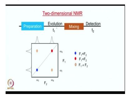
This is two dimensional NMR and this is based on the concept of segmentation of the time axis and the time axis is separated into 4 periods like this to the preparation period and then you have the evolution period  $t_1$  and the mixing period, then you have the detection period  $t_2$ . These are time variables which means you will do lots of experiments, a series of experiments varying the values of  $t_2$  and the data is collected as a function of time during the detection period  $t_2$ .
