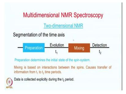
The basic concept of two-dimensional NMR as I mentioned to you is in the segmentation of the time axis. This is called the segmentation of the time axis. Here we have the time axis and now you actually divide this time into 4 different periods. I will explain this to you what these one periods are and just to take note of this, this is the so-called one preparation period, then this is followed by an evolution period then a mixing period and then detection period.
