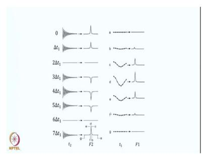
So here is a actual demonstration. Here you have the first data point, time t=0. You have the first FID, and then  $\Delta t_1$  you have the second FID. The third  $2\Delta t_1$ , this is the third FID but there is no signal here. As, I said there will be modulation and depending upon what the initial point is, and how the system evolves, what the signal is present, you will have these different kinds of FIDs so each of these FIDs is different.
