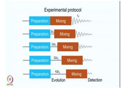
Now, so how is the experiment actually performed? Experimental protocol is given here. So you do a series of experiments. In other words you collect series of FIDs. Typically the data you collect is in the form of FID and that happens in the  $t_2$  period. So, here you have the preparation period and the evolution time here, it is 0. So we call it as zero time period here, and is immediately followed by the mixing and you collect the data as a function of time  $t_2$ .
