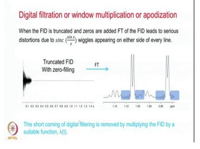
And there is more exclusively indicated here you have truncated FID with zero filling the you get this wiggles here, these are the form of sink or the  $\frac{sinx}{x}$  wiggles appearing on either side of your lines and this is not desirable.
