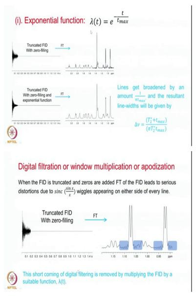
So the first thing that one could do is multiply by an exponential function which is of this form, window multiplication, digital filtration or all the three term means the same thing, okay? Different times we use different terminologies. So you multiply an exponential function, exponential function is given by this manner
