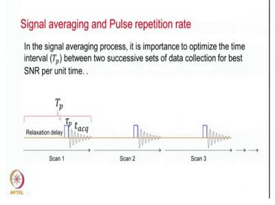
The next point to consider is signal averaging and pulse repetition rate, we say signal averaging is easy in the case of Fourier transform NMR because you can improve you collect the data for a very short period of time and you can repeat this process so you can increase your signal to noise ratio.
