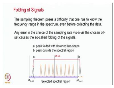
So, the sampling theorem therefore possess its difficulty that one has to know the frequency arrange in the spectrum, even before you collecting the data.
