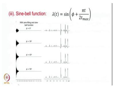
Sometimes we want to use a function of a different type which is called as a the sine bell function, the sine bell function has a this sort of a formula this is
