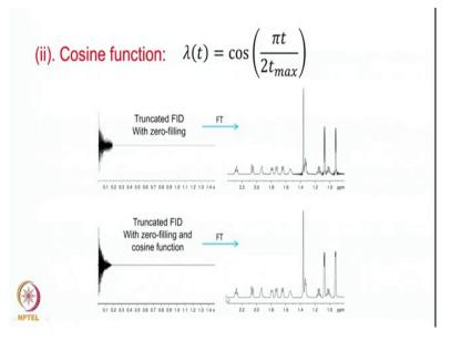
Then you have other functions, the next function which is commonly used is cosine function when you do the cosine function you multiply your FID by such a kind of a function. So this will be a function which adjusted in such a way that you start from here the 0 point is here and it will slowly come over and come to 0 at this point, okay?
