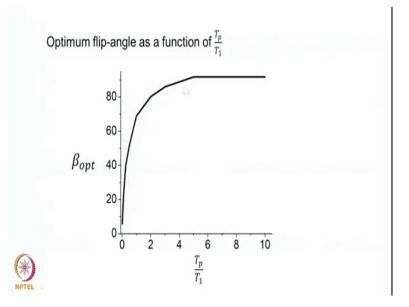
And this same curve if plotted in the different style your plot the  $\beta_{opt}$  verses  $\frac{T_p}{T_1}$  and you can see here for very large T1's you need to have actually optimum value of flip angle is given by this manner, so you have  $\frac{T_p}{T_1}$  is very small then your optimum flip angle is here and  $\frac{T_p}{T_1}$  is very long then you have an 90° flip angle, okay?
