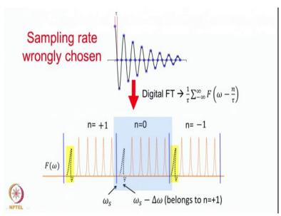
So what is the consequence of the digitization theorem? Sampling rate is wrongly chosen, as I mentioned to you earlier, we placed the offset somewhere and we chose your spectral width wrongly and then you collect the digitized data in this manner and do it digital Fourier transformation then it is consequence of this digital Fourier transformation that you get lines to fold.
