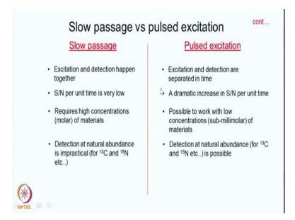
So a consequence of this is the following, excitation and detection are separated in time in pulse excitation, whereas, here excitation and detection happen together, what I mean excitation and detection are separated in time we apply an RF and following the RF we detect the signal as an FID.
