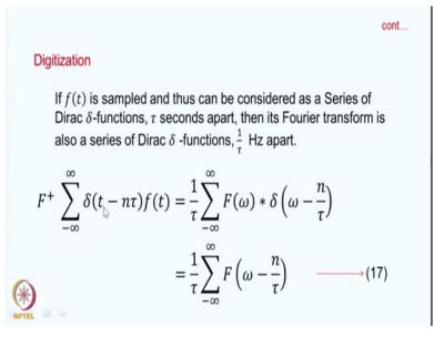
Digitalization means that your FID is an analog signal it is a continue signal which is coming as in this manner, but we collects the signal in a continuous manner. Suppose, we were collect the data as a series of Dirac  $\delta$  function, the words we collect the points at certain time
