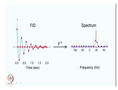
So this is schematically indicated here for your easy understanding, this FID was like this we are not collecting the FID in this manner, we collect the FID as a series of points and the time between two consecutive points is tau this is called as a dwell time and this is also represented as sampling. So, how you sample your FID? You collect the data here, a point here and a point here and a point here and a point there.
