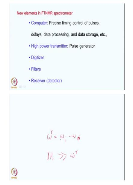
So if have to summarize this in words, you have the computer control is essential, precise timing control of pulses, delays because you need to know how much delay you have given because we see the delay equalization leads through phase modulation of the spectrum and therefore, you need to know how much delay you have put and we should be precise and we need to know exactly how much is that? Data processing, and data storage, etc.
