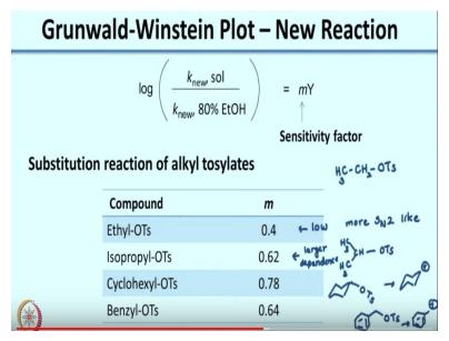
So to do that you use the Grunwald-Winstein plot. And here what you have is you have log of k new which is your new reaction, not your t-butyl chloride in your unknown solvent divided by k new in 80% ethanol and you compare that with Y which you get from the t-butyl chloride reaction. So this is exactly like what we had seen in the Hammett case.
