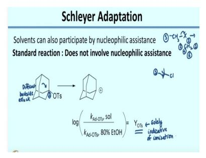
So what is meant by nucleophilic assistance is if you have and this is the solvent, the solvent might participate in some sort of a backside attack, which would help in the process of ionization. So what you end up getting would be, which is further stabilized by solvation. So now one would not expect much of nucleophilic assistance for the t-butyl chloride dissociation.
