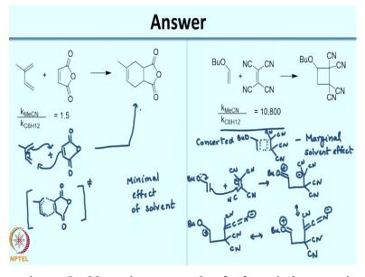
So the first reaction as I told you is an example of a four pi plus two pi cycloaddition reaction also called as the Diels-Alder reaction. Now the Diels-Alder reaction is a concerted reaction. What that means is you do not have an intermediate, what you essentially have is a cyclic transition state. It comes under a class of reactions called as pericyclic reactions. And if I were to draw the mechanism for this, so the mechanism would look like this.
