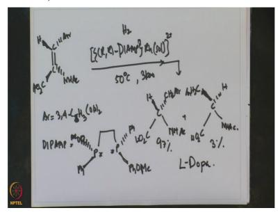
Is Ar, hydrogen, C, NH, AC, C, O 2 H. Ar = 3 4 C 3 C 6 H 3 OH whole 2. DIP AMP = O Ph O Me, phosphorous, Ph. This is a chiral entity. P, this phosphorus is also chiral; Ph, Ph O Me. So, this is the DIAMP ligand. And this is used for preparation of L-Dopa which is R R DIAMP rhodium Sol 2 + 50 degree centigrade 3 bar in presence of hydrogen, gives a highly 2 isomers in highly enantiopure form; CH 2 Ar, N H Ac, C O 2 H and H.
