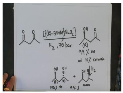
1 3 diketone reacting with R BINAP Ru Cl 2 in presence of hydrogen 70 bar gives alcohol R 99% ee at 10% conversion. And which, if allowed to react more with hydrogen then; so, the first obviously is the reduction of the diketone to alcohol and a ketone. So, one of the group that reduce the other chelates, but if one continues with the hydrogenation, then both the carbonyl compounds are reduced to alcohol.
