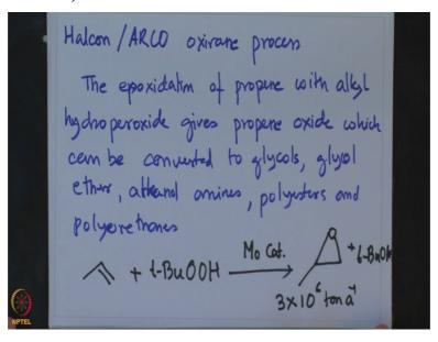
So, as one observes that Halcon/ARCO oxirane process is really an important process because this is a industrial scale epoxidation process of propylene with alkyl peroxide. Hydroparoxide in presence of a molybdenum catalyst that gives these propene oxides. Now this propene oxides are important intermediates for accessing glycols, glycol ether, alcol alconol amine, polyester, polyurethanes and etcetera.
