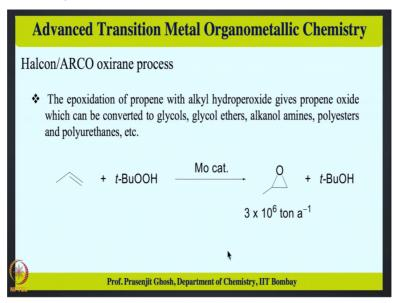
So, we sort of take up this new reaction which is new epoxidation reaction which is called Halcon/ARCO oxirane process.
