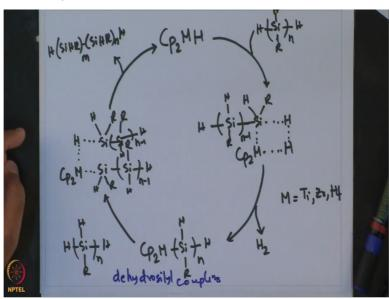
So, this is the Cp 2 M H where are the 2 cyclopentadienyl ligand. And then, the first reaction is the addition of the silyn H, Si, H, R, H. This silyn comes and adds and form a 4 membered sigma bond transition state. So, this is given as Cp 2 M, H, Si, H, R, H, then Si, H, R, H, whole n-1. And these, since it is dehydrogenative coupling loses hydrogen this hydrogen H 2.
