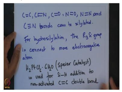
So, this is kind of very interesting information that hydrosilylation can be done on C-C, C-N, C-O, C-O, N-O, N-N, C-N and C triple bond N, can be silylated. For hydrosilylation, the R 3 Si group is connected to more electronegative atom. So, in this case, for C-N the Si 3 R 3 Si would be on nitrogen; for C-O the R 3 Si would be on oxygen and hydrogen will be on carbon, is same over here. For N-O R 3 Si will be on nitrogen and C-N R 3 Si will be on nitrogen.
