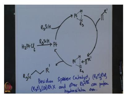
H 2 Pt Cl 6 in presence of R 3 Si H giving platinum 0. And this platinum 0 then oxidatively add R 3 Si H to give this platinum based sigma complex of the type Si R 3 and then to this olefin R dashed attacks to give this olefin bound complex. Olefin attacks from the external side Si R 3, R dashed to give the corresponding product which is R dashed Si R 3 along with the regeneration of the platinum 0 species.
