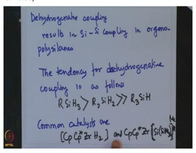
So, dehydrogenative coupling results in silicon-silicon coupling in organopolysilane. The tendency to, towards degenerative dehydrogenative coupling is as follows. The tendency for dehydrogenative coupling is as follows. Which is, R Si H 3 R 2 Si H 2 > R 3 Si H. And the catalyst used in this cases are mixed CP type, very interesting catalyst. They are the catalyst
