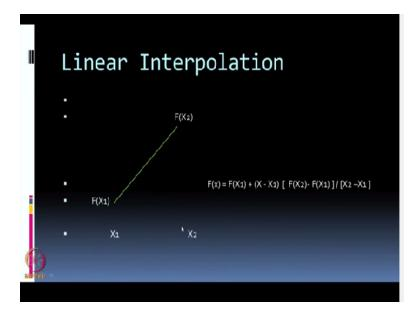
This particular slide demonstrates what is linear interpolation. x1 and x2 are the points on the x axis and this line is a line that has values fx1 at x=x1 and fx2 at x=x2. So between these 2 points, I do not have any data. And I want to interpolate using a straight line that is for all values between x1 and x2, I want to say that the function is a straight line and I want values of fx at those points.
