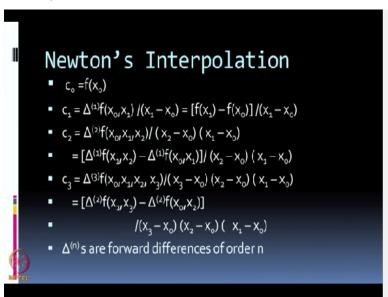
The formula is given here. This is the Newton's interpolating formula. We also call it a forward interpolation. Forward interpolation because you will go from x0 to x1, x1 to x2 and so on. So my C0, the first constant is the value of the function at x=x0, okay. So this is my C0. C1 is given by delta 1fx0x1/x1-x0. Now this delta 1fx0x1 is called a forward difference. What do I mean by the forward difference?
