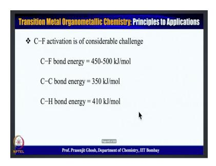
C F in the tune of C C and C H bond activation T C F bond acceleration probably is by far; the most difficult to achieve with c f bond energy between 400 to 500 kilojoules per mole.
