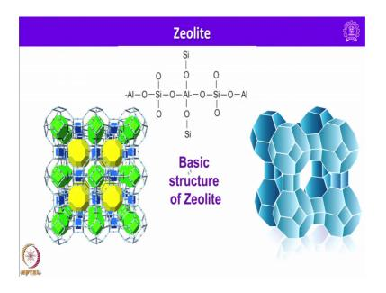
So this also this one unit we call it as sodalite structure, this how the cages in zeolite look like.
