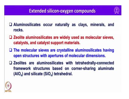
Occur naturally as clays minerals and rocks and zeolite aluminosilicates are widely used as molecular sieves catalyst and catalyst support materials. The molecular sieves are crystalline aluminosilicates having open structures with apertures of molecular dimensions and zeolites are aluminosilicates with tetrahedrally connected framework structures and based on corner sharing aluminate Al O 4 and silicate SiO4 tetrahedras.
