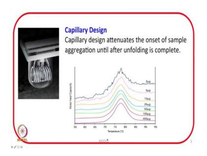
This is a design which is capillary design and you can see the cell will have one inlet and there will be another outlet; that means, you can sell fill the sample from one side and it can go through the capillary fill the cells and it can come out from other side.
