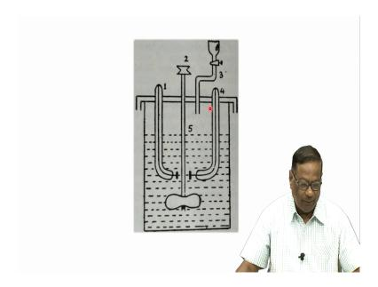
So, like this the electrodes are; the electrodes are mounted like this, here you see my pointer that is one electrode, another electrode is here, I have a stirrer and then 2 these are the wires fused in a glass. So, that wires are not directly exposed to the aqueous solution, only this part of the wire is exposed in their solution, here is my burette a very simple arrangement nothing very complicated about it.
