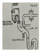
A low velocity jet of air impinges on a dilute solution of hydrogen peroxide contained in a conductivity cell. The gas is not only absorbed, but the jet induces rapid microcirculation that provides adequate mixing of electrolyte. The peroxide oxidizes the sulphur dioxide to sulphuric acid in the interim.
