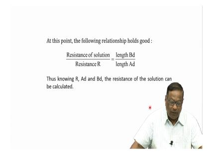
So, at this point resistance of the solution and resistance R are exactly equal to length Bd and Ad, ok. So, knowing; we know R, we know Ad, we know Bd because this can be measured it is there just part of the 1 meter wire one half length this is one side this is other side. If we know one side where the sound is minimum, the other side is automatically fixed. So, we know three parameters in this equation. So, resistance of the solution we can calculate.
