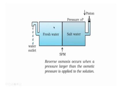
Now, imagine here I am drawing a picture of reverse osmosis and this is a SPM; semipermeable membrane and I have put salt water and osmotic pressure is there and I have a; I put pressure on this solution and fresh water is; it is allow fresh water on the other side ok.
