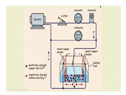
Now, this is a sort of figure for you to study the operation of an electroplating bath. Here I have a sheet copper anode ok and here I have sheet copper anode again and then this is the work to be plated with the copper solution; that means, I have one cathode and two anodes ok. Center one is cathode and this is anode so, that copper sulfate copper from the anode can dissolve and come over here and then get plated and then the article will be plated with copper.
