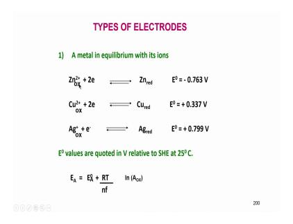
So, here I have a zinc metal, I have a zinc metal in the oxidized state ok, that is carrying plus 2 charge that can react with 2 electrons, it can pick up 2 electrons and become zinc metal that is reductant.
