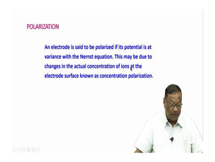
So, an electrode this I have already explained to you that in electrode is said to be polarized, if it is potential is in variance. But now we are talking about the potential not the voltage and we are talking about the electrode.
