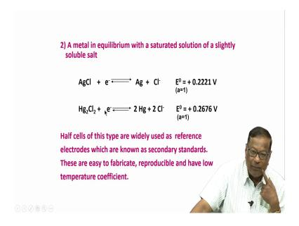
So a metal has ion, that is one kind that is a metal in equilibrium with it is own solution ok, in equilibrium with it is own solution a metal to wire rod electrode in equilibrium with it is own solution couple to standard hydrogen electrode.
