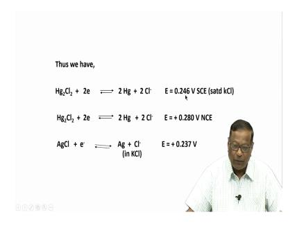
Third one is we can prepare this half cell you know before I go to the third one, we can have 2 types of reactions with respect to Hg 2 Cl 2, that is I can write something like this; Hg 2 Cl 2 plus 2 electrons goes to 2 Hg plus 2 Cl minus that goes to 0.246 versus saturated kCl electrode. This is a reference electrode now. This saturated kCl saturated calomel electrode it
