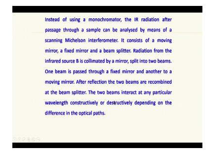
So instead of using monochromator the IR radiation after that passage through a sample can be analyzed by means of a scanning Michelson interferometer. This is a sort of again second year PU physics material that is interferometer they start around that level, basically it consists of a fixed mirror, moving mirror, beam splitter etc. So radiation from the infrared source is collimated by a medicine already told. I have only putting it here for the record.
