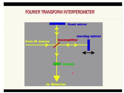
IR source I have been splitter, I have moving mirror, I have fixed mirror, beam splitter splits into 2 and then fix a mirror reflects, the moving mirror also reflect. All the reflected radiation is passing through the sample and goes to the detector whatever is the remaining that is on except IR.
