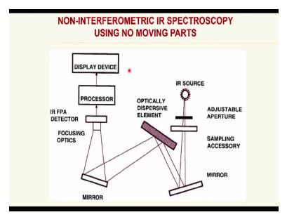
And it producers a IR spectrum here, so non interferometric IR spectroscopy, this is the typical optical arrangement ok I have IR source here and then adjustable aperture is basically a split is and then a sampling accessory, I have a mirror and this is the grating, this is non FT-IR. So grating is here and all the radiation from the grating is collected on to the mirror and it is focused and then IR-FPA detector is here.
