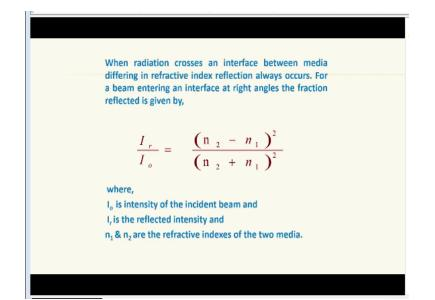
When radiation crosses an interface between media differing in refractive index reflective index reflection always occurs. This you should understand, so the radiation crosses an interface between 2 different media we can always imagine radiation passing through an air and then passing through a glass mirror or a glass block or a plastic block and then coming out. So, that is what we have talking about.
