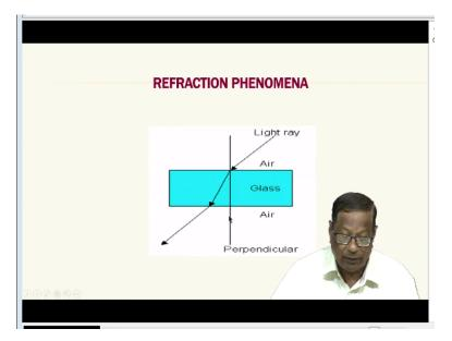
So, refractive phenomena I can always show like this that it is this is a block of glass and then radiation is coming like this. This is the perpendicular to the glass and then it comes here, changes direction and then again comes out of this thing that means if they changes were not there. If the glass was not there it would I have travelled like a straight line, even though we say that it is wave electromagnetic radiation travels in waves etc. in simpler terms for practical purposes.
