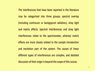
Sometimes stray lights is also introduce it is interferences and matrix effects. So, we have already discussed matrix effects quite a lot and spectral interferences and stray light interferences relate to the spectrometer whereas, matrix effects are closely related to the sample introduction, and sample excitation part of the system. So, the causes of these different types of interferences are very complex.
