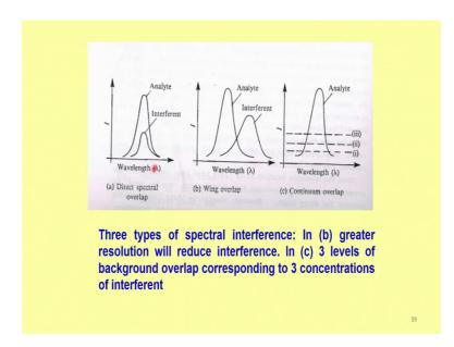
So, here I am showing you some of the interferences spectral interferences. You can see part a here the interferent is there analyte is here on the above, but you have to your suppose to subtract this the interferent this much of emission said to be subtracted from the total area of the analyte. Here it is the spectral system interferent is totally inside the emission spectrum. So, this is known as direct spectral overlap.
