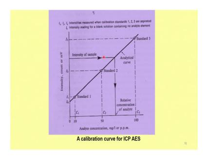
So, this is how we do the plot here I plot intensity or count on my count or millivolts that is the photon response and analyte concentration is here on the x axes; that is 10 p p m 50 p p m 100 p p m. I told you this is order will be it will be linear over several orders. So, write from 0.0 write from 0 p p m I can go up to 1000 p p m also depending upon.
