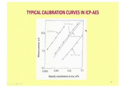
Here you can see that the I am showing you the first one is vanadium ok. Hm this is analysis of metals in iron that is weight percent. So, we have analyzed titanium using 334.94 nano meter you can see the plot of concentration from 0.00 0001 up to 0.00 that fall somewhere here up to 0.02 or something like that ok.
