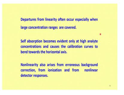
So, do we have always a linearity? Answer is no because linearity is always expected for very low concentrations normally, but the whenever large concentration ranges are covered we do see some departure from the linearity when; that means, the counts will not be exactly proportional to the concentration.
