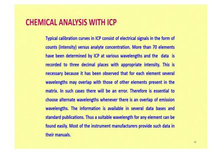
So, it is important for us that other elements should not interfere with the determination of other elements our analyte, because many emission lines still match with the analyte element.
