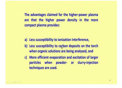
On the torch when organic solutions are being analyzed because hardly carbon will deposit whatever carbon is there it will just burn off and so the carbon deposits due to organic solutions are very less and efficient evaporation and excitation of larger particles, when powder or slurry injection techniques are used these are the some of the advantages ok.
