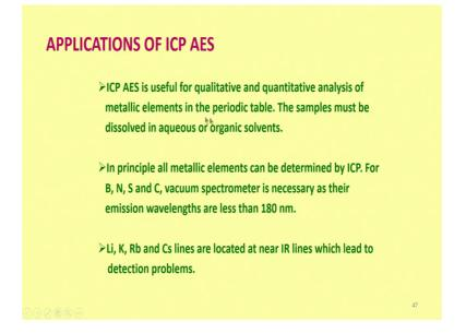
So, the applications of I a s ICP AES now I am talking only about ICP AES not DCP AES also. So, it is useful for qualitative and quantitative elements this is like your university examination. If I say list the advantages of ICP AES you should write this, ICP AES is useful for qualitative and quantitative analysis for this samples must be dissolved in aqueous or organic solvents.
