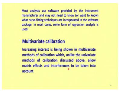
So, most of the analysts use the software provided by the instrument itself. Normally, whenever you do the chemical analysis and the data is generated the computer software ask you do you want to fit the data into linear curve or quadratic curve or polynomial? So, you can choose, look at the apply all the three and see which one looks better the calibration curve which one looks more linear. So, that is possible and it is also important that some sort of regression analysis is used.
