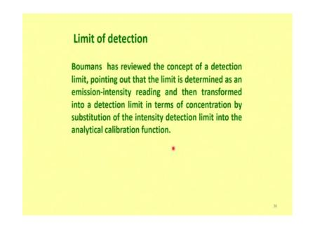
Now, I want you to understand that another concept that is limit of detection. So, what is the limit of detection? So, far we are discus sensitivity. Sensitivity refers to the method ok, sensitivity refers to the method where the signal is measured with respect to concentration. Now, what is limit of detection then? That is, the sample which we can say with confidence that yes there is a sample the sample analyte is there in a given sample.
