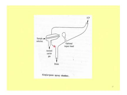
So, then we have a single pass spray here, what is happening, the sample is coming here, aerosol is carrier gas is coming it is going to impact the bead that is fixed here. So, again because of this kind of design, whatever are the heavy droplets will slide down slowly, and then fall into the drain, and only the aerosol will be going up. So, this is a single pass spray chamber, different types of nebulizers are always there.
