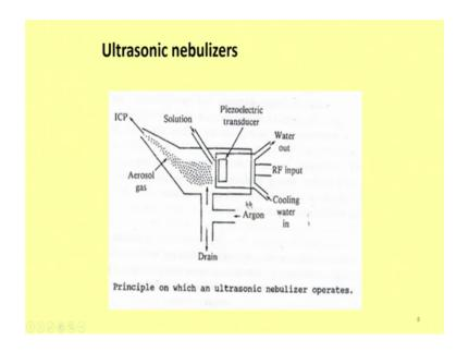
This I had shown you knew, this is the ultrasonic nebulizer, we have a piezoelectric transducer solution coming here, hits it and then goes into forms an aerosol, and bigger droplets fall into the drain, where as argon is coming from the side ok.
