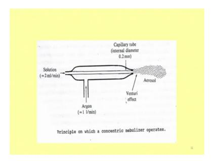
So, this is a concentric nebulizer system solution is coming here, approximately about 2 m l per minute, and then capillary tube is here, 0.2 mm, argon comes here venturi effect, and then this argon will going it pulls the liquid also, and an aerosol forms ok.
