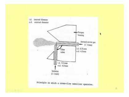
This is more tolerant with the dissolved solids. Suppose you want to determine the iron content in blood, or thallium in blood, or lead in blood. So, most of the samples contained dissolved solids, quite large quantities, sometimes if it is a seawater base you would know that the salt content would be approximately 3.5 percent that is 35000 p p m, and in that you want to determine few elements at p p m, 1 p p m, 2 p p m like that.
