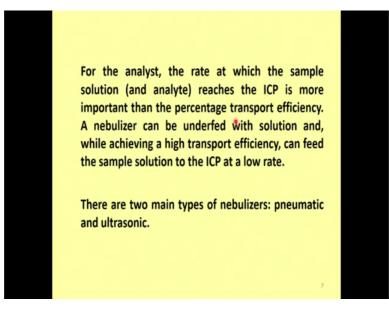
So, a nebulizer can be underfed; that means, it should be starred with solution, and while achieving a higher transport efficiency, it can feed the sample solution to the ICP at a low rate there are two types of nebulizers one is pneumatic another is ultrasonic. So, as I explained to you ultrasonic is a special equipment by itself, you have to buy whenever you want to buy an ICP instrument here, to buy the sample nebulizer also.
