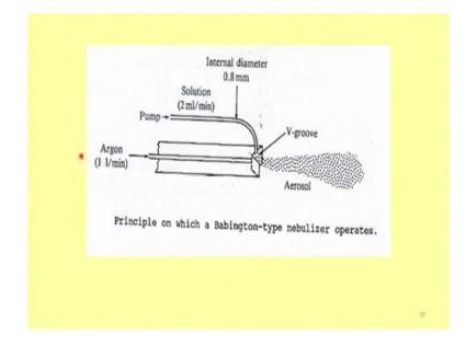
So, this is the Babington type nebulizer here, we have an argon sample and a solution is coming here, there is a wedge here ok. This gas passes through, this wedge sample comes into the wedge from there, because the gas is moving, and because of the Bernoulli effect the aerosol is generated.
