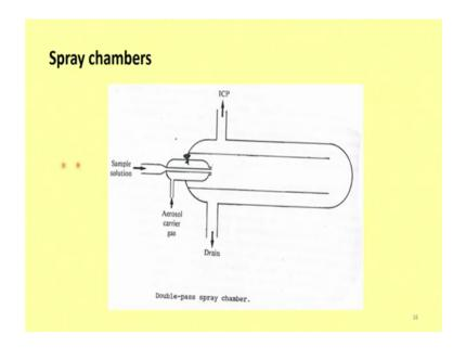
So, spray chambers are essentially, what is a spray chamber is a box in which aerosol carriers sample solution, and everything is held there, and part of the it is arranged in such a way that the aerosol gets carried up upwards, and the bigger droplets fall downwards. So, that is known as a spray chamber look at this slide.
