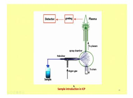
And then, we have, there are ways of introducing the sample. So, what I have here is, I have the sample, a sort of a peristaltic pump, it gets sucked here, and then into the nebulizer, Argon gas is there, a fine mist is generated, bigger droplet us are collected back into the drain, and then the final droplets of the order of about 10 micrometers get carried into the plasma torch, which enter the, into the plasma, and then the emitted radiation must pass through the grating and detector.
