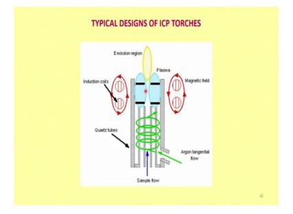
That 3 concentric circles in which the Argon gas is flowing, it is flowing round and round also, its sample is picked up like this, and then it enters the system.
