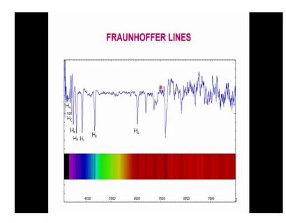
I will show you what is a Fraunhofer line, here you can you can see that solar spectrum contains dark lines like this is intend of the intensities. So, we initially intensity is very high suddenly there is a dip and then again a there is dip again it goes up again it goes in a steady, again it goes down like these we can see the whole solar spectrum. But if you take a photographic plate this is the energy figure drawn.
