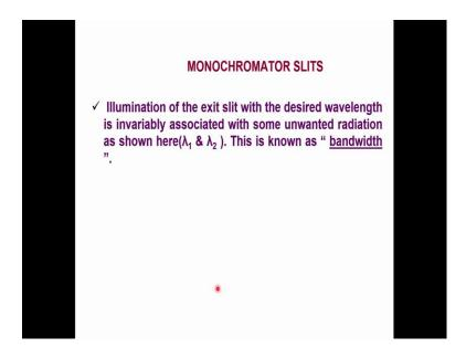
So, illumination of the exit slit with the desired wavelength is invariably associated with some unwanted radiation as shown here I want to show you in the next slide; normally what happens is look at this figure once again any rectangular slit here will also pick up some unwanted additional wavelengths nearby. You know you will never get a true monochromatic radiation.
