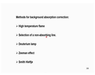
What are the different methods for background correction? Now you are imagine that we are discussing the background absorption it is an interference in atomic absorption and background absorption must be corrected before we actually take the absorbance from the analyte.
