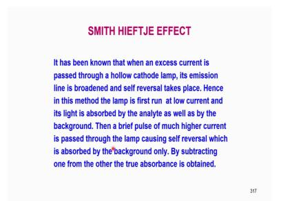
In Smith Hieftje self reversal takes place and lamp is first run at low current and then a high current. So, whenever there is high current there is no absorbance and only the background will be checked and a brief pulse of much higher current is passed through and we subtract the sample from the background.
