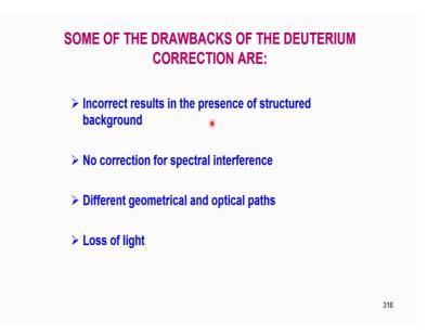
So, now deuterium correction background there are advantages and disadvantages. So, the drawbacks include incorrect results in the presence of structured background occurs and then no correction for spectral interference nothing can be done and different I accept go for some other resonance line here in the second one.
