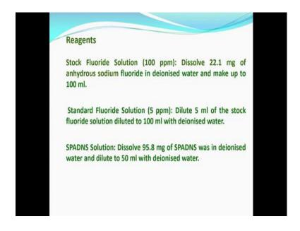
So, the principle of this method is that the fluoride this complex SPADNS reaches reacts with zirconium to form a red dye. I can give you the structure of this.
