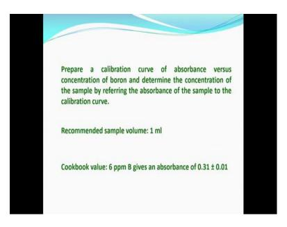
If I say recommended sample volume is 1 ml it means it is only a recommended sometimes if the boron concentration is lower you can take higher concentration also, but remember that the final volume should be 10 milliliters only.
