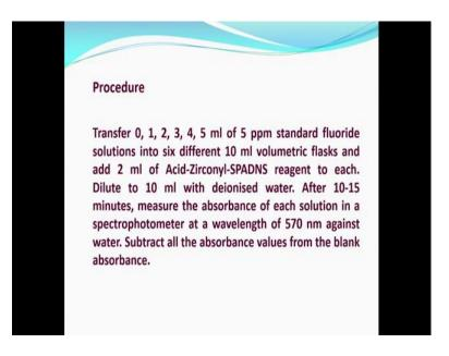
Now, what you should do is the go for the procedure once you have all these things ready. What you should do is transfer 40 to 5 ml of 5 ppm of fluoride, and different volumetric flasks add the reagent 2 ml and then dilute to 10 ml. After about 10 to 15 minutes you see here again I am saying 10 to 15 minutes for the reaction to complete if you do not do it you may not end up with a stable result.
