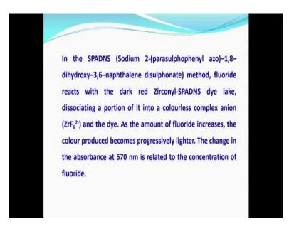
So, we can look at it from the analytical point of way how do we go about doing the analysis of fluoride. The chemical analysis of fluoride is normally accomplished using a reagent called as sodium 2 parasulphonyl azo 1 3 dye hydroxyl 3 6 naphthalene disulphonate.
