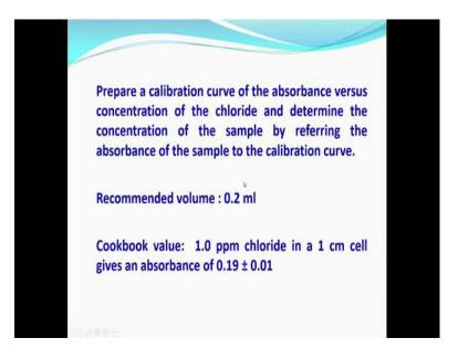
And cookbook value is 1 ppm of chloride that is a standard in 1 centimeter cell should give you an absorbance of about 0.19 plus or minus 0.01 ppm.
