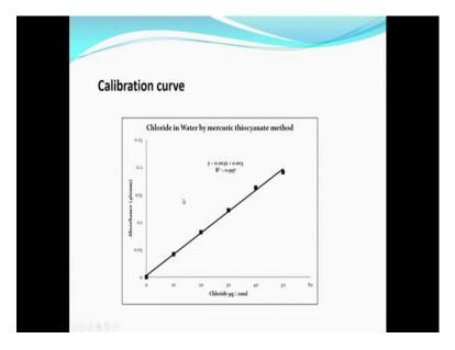
So, this is the calibration curve you can see that the linearity is given by y is equal to 0.003 x plus or minus 0.003 this refers to intersection very less. So, it must pass through the origin, and the concentration the linearity the slope is 0.997 almost one therefore, it is approximately at 45 degree angle to the sample.
