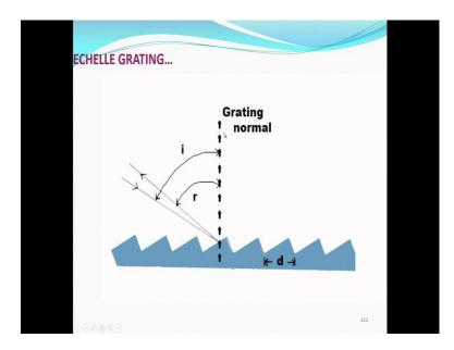
And then what happens is this the difference is like this this is normal grating normal, the angle of incidence is fixed and angle of this thing is reflection is also fixed like this this is the distance between their to.
