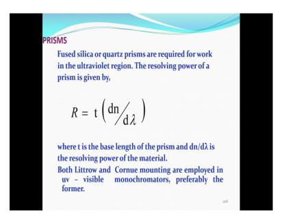
So, prisms apart from lenses and monochromators glass filters, we use prisms and prisms we have discussed earlier fused silica or quartz prisms are required, silica prisms are required for the visible range and quartz prisms are useful for the ultraviolet range.
