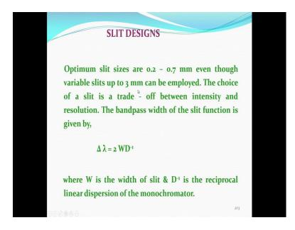
Basically what is a slit? A slit is a simple material a metal plate in which a hole is made that is a slit. I take a metal plate and make a small hole through which the radiation is coming. So, I put. So, I take the radiation source on the left side and then put a metal plate so that nothing comes out and all the radiation that is coming out will be only through the slit, and the slit designs are normally in the form of triangles.
