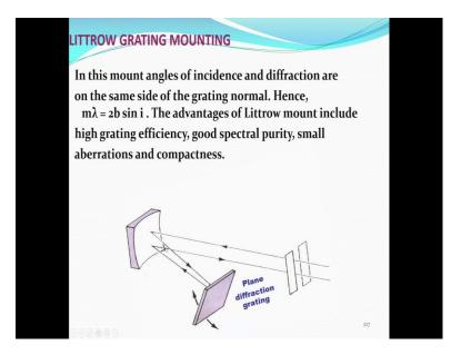
So, another arrangement is this is Littrow single entrance slit and exit slit, the difference is entrance slit is coming from the top and exit radiation is also is also coming through the same slit, but slightly at a lower level. So, this is known as Litrow grating mounting. So, there are the if we advantage of this is high grating efficiency, good spectral purity, small aberrations and much more compact then double slits very simple arrangement.
