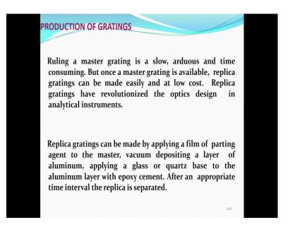
Now, how do I produce a grating? A grating is produced using a master grating once you know every time it is not possible to get the same quality of grating, by taking a machine and doing it. So, what we do normally is we take a master grating make a master grating and then produce there replicas. So, basically it is a slow arduous and time consuming, but once a master grating becomes available replica gratings can be made very easily and that to at low cost.
