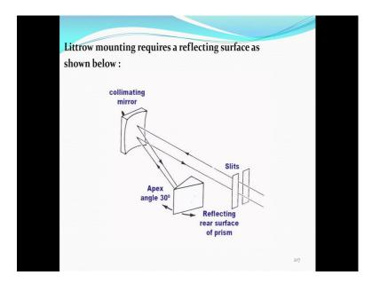
Now, the prisms there is an arrangement, typical arrangement I am showing you now here is the slit and from the slit I get a parallel radiation, here it is a collimating mirror and from the mirror the radiation is reflected back to a prism either it may be Littrow or Cornue mounting and the whatever radiation comes out should go should be a monochromatic radiation useful for measurement.
