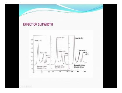
And here the peak things are normally you can see the sharpness of the peaks as the bandwidth varies from point 3.4 nanometer slit width is 1 nanometer this is 0.5, and this is 0.1 millimeter. So, here bandwidth is more 0.34 band width is well one plus I here it is 0.7 and it is 3.4 nanometers. So, you can see the peak heights entirely different for the same system.
