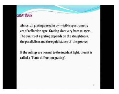
So, next thing is gratings; gratings are better than prisms to choose the correct wavelengths, almost all greetings are used in UV visible spectrophotometry are of reflection type; that means, the gratings are coated from the bottom so that the radiation that is falling simply gets reflected and grating size is varies from 10 to 25 centimeter the quality of a grating depends on the straightness parallelism and equidistance.
