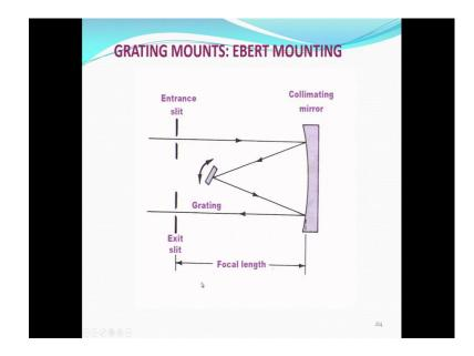
So, what I had told you so far is I want you to concentrate now the radiation that is normally I am coming from the radius from a spectro from a radiation source like tungsten lamp or something, that has to pass through a slit and then a monochromator a lengths or something to make the lines parallel.
