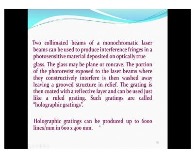
So, two collimated beams of a monochromatic laser beams can also be used to produce interference fringes on a photosensitive material, deposited on optically true glass.
