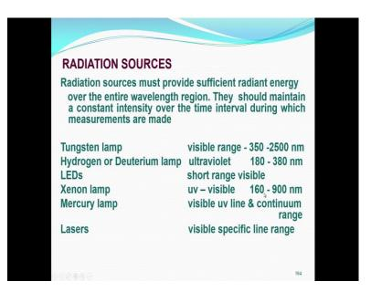
So, what are the radiation sources? So, I have a number of choices, depending upon the concentration, depending upon the cost and depending upon the sophistication I want. Normally radiation sources provide sufficient radiant energy over the entire wavelength region; that means; in spectrophotometry what I need is a lamp which gives light in all wavelengths.
