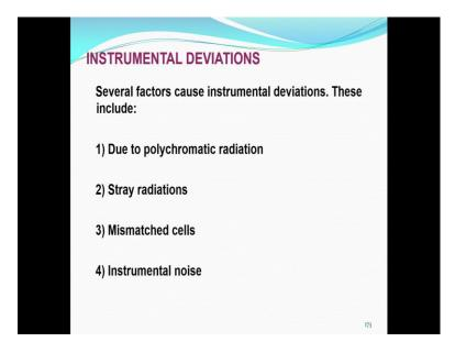
And then in instrumental deviations we have polychromatic radiation problem, stray radiation, mismatch cells and instrumental noise etcetera, and then we had also discussed the deviations for effect of bandwidth and slit width.
