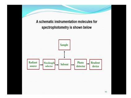
So, a schematic representation of the molecules for spectrophotometry is like this, I need a radiant source that is here and then I need a wavelength selector, I need a sample solvent; solvent is for reference, sample is for measurement. So, these two are interchangeable and then I need a photodetector and I read out device these are the basic components.
