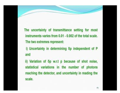
The basically the uncertainty of transmittance setting for most instruments varies from 0.01 to 0.002 percent of the total scale.
