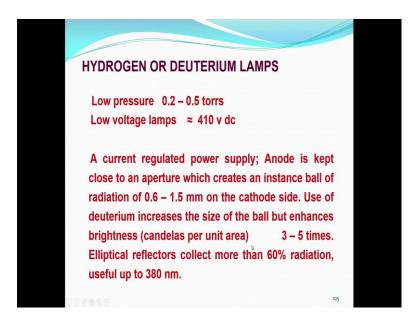
So, containing our discussion hydrogen lamp or deuterium lamp, so it is a low pressure lamp; that means, drival pressure in the lamp is only 0.2 to 0.5 torrs, it is a low voltage lamp also 410 volts and a current regulated power supply is required to generate; why because what we normally get is 220 volts dc.
