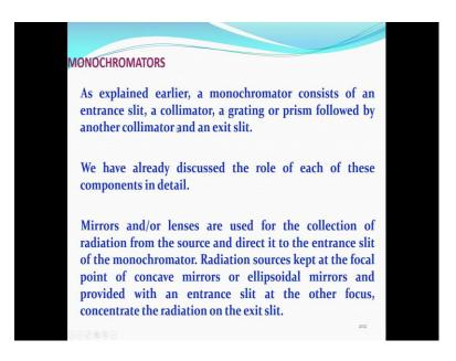
So, monochromators it consists of an entrance slit, a collimator, a grating or prism followed by another collimator and exit slit. We have already discussed the role of each of these components in detail during the general discussion.
