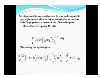
So, the minimum relative concentration error for most modern uv-visible spectrophotometers, where shot noise predominates we can show that d T is proportional to the square root of the radiant power. So, I put these numbers and then differentiating this equation again I get a multiplication term another multiplication term and then 1 over 2 this should be 0.
