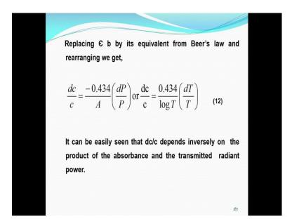
Now replacing epsilon b by its equivalent from Beer-Lamberts law, what I get is dc by c is equal to 0.434 divided by A of d P b y P or dc by c is equal to 0.434 d T by T this is in terms of transmittance the first part is in terms of power. So, we can see that dc by c depends inversely on the product of the absorbance and the transmitted radiant power.
