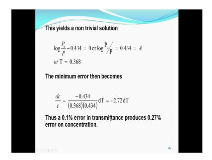
So, log of P naught by P is equal to 0.434 that should be equal to 0 or log of P naught by P is equal 0.434 which corresponds to a transmittance of 0.368.
