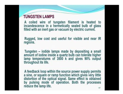
So, tungsten lamps again as I was telling you a coiled it is just a small bulb which you would have a seen in your day today life, it contains a coiled wire of tungsten or nickel or something like that, and then it is heated to incandescence in a hermetically sealed bulb; that means, no not high pressure lamp and then it is filled with in either inert gas or a vacuum or by vacuum and it is heated by electric current.
