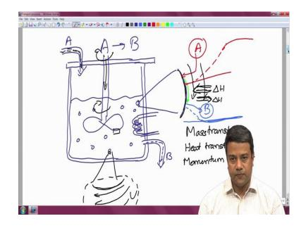
And we looked at the mass transfer from the surface, the heat transfer to the surface and so on when we consider a single particle and we saw how the dependent variable can be described in terms of dimensionless groups. The dimensionless flux has a function of other parameters the Reynolds number and Prandtl number or the Schmidt number.
