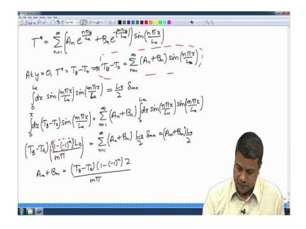
The solution that I had for the temperature; field summation n is equal to 1 to infinity A n e power n pi y by L x plus B n e power minus n by y by L x into sin of n pi x by x and the inhomogeneous boundary conditions are that at y is equal to 0; T star is equal to T B minus T naught. Recall that at y is equal to 0, the value of T star is equal to T B minus T
