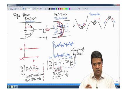
There are velocity fluctuations in all directions, there are eddy velocity fluctuations correlated parcels of fluid that are in correlated motion. So therefore, a turbulent flow is inherently unsteady and it is inherently three dimensional. The velocity fluctuations are not only in the flow direction they occur in all three directions. And these velocity fluctuations or these correlated parcels of fluid they transfer momentum far more efficiently than the transport due to molecular diffusion.
