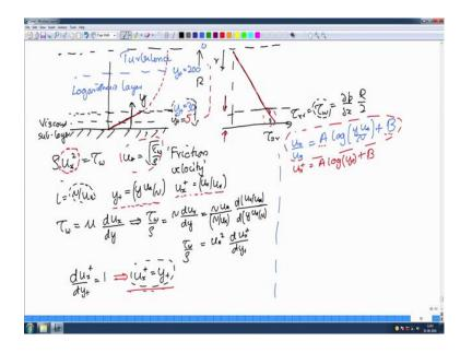
So, I had shown you that for a turbulent flow the bulk of the flow.
