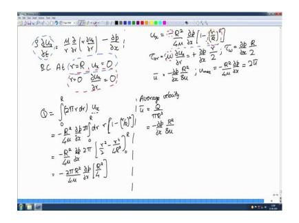
So, this will be equal to minus r square by 4 mu delta p by delta x integral 0 to r of dr into r into 1 minus r by r whole square, and I have an additional factor of 2 pi here 2 pi is just a constant. So, I have integral of r square minus r; I am sorry integral of r minus r to the 4. So, this will be equal to minus r square by 4 mu dp by dx times 2 pi into r square by 2 minus r power 4 by 4 r square between 0 and r. So, that is what I get by doing the
