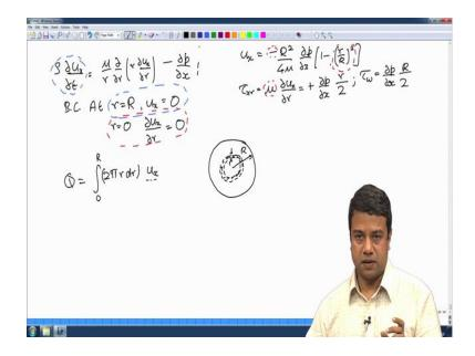
At the wall of the pipe the shear stress tau w is equal to dp by dx into r by 2 mu; I am sorry there should be no viscosity there because I multiplied by this viscosity here. When
