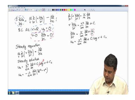
So, let me write that once again for you the total momentum conservation equation for a general unsteady flow has to be of the form mu by r d by dr of r d u x by dr minus dp by dx, so that is the momentum balance equation. First we consider and the boundary conditions at the surface of the pipe r is equal to r u x is equal to 0 and at r is equal to 0;
