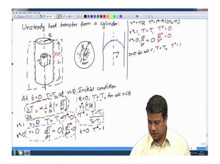
And we had derived differential equations for that; the distance from the axis of the cylinder was the co-ordinate, the second was the distance along the axis that we had assumed that there is no variation in that second direction and we had got an equation for the temperature field.
