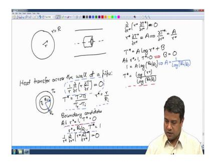
We had solved the heat transfer across the wall of pipe, the study problem and we have got the logarithmic profile for the temperature field which is different from the linear profile you would expect if you had for transport cross flat surfaces.
