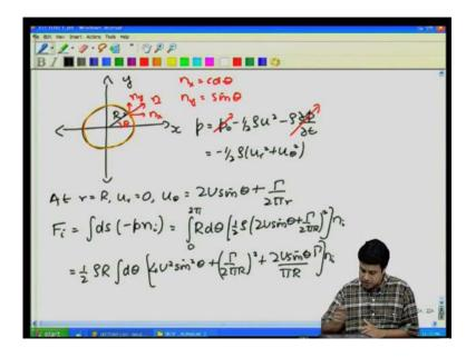
So, we want to calculate the force on the cylinder cylinder with radius R x and y the unit normal to the cylinder at the surface n has two components n x and n y. The angle theta the angle theta if I have n x will be equal to cos theta, n y is equal to sin theta how do I calculate the force, first I calculate the pressure from that I integrate over the surface to get the force. So, the pressure is given by p is equal to p naught minus half rho u square minus rho partial pi by partial d.
