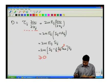
So, that is the energy balance equation as I said it is only for the mechanical energy balance equation, so whenever if you want to estimate how much heat is generated due to the fluid flow the desperation rate in the fluid is basically going to be equal to tau i j times partial u i by partial x j. So, this completes our derivation of the of the conservation equations the constitutive relations the boundary conditions, and I talked briefly about energy dissipation.
