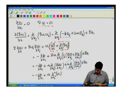
To write it out in detail once again the mass conservation equation is just that partial u i by partial x i is equal to 0 or divergence of the velocity is equal to 0, the momentum conservation equation I can write in two ways partial of rho u i by partial t plus partial by partial x j of rho u i u j is equal to partial by partial x i of minus p and I should take j here delta i j plus 2 mu E i j plus rho a i.
