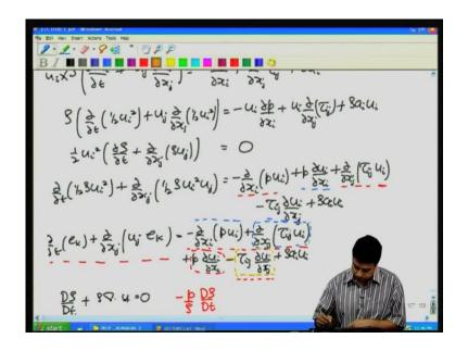
So, therefore, this represents the irreversible dissipation of energy, the conversion of mechanical energy into heat and that is appearing as you can see here, in this equation that conversion is appearing as a sink term, in the mass conservation energy conservation equation. It always tends to reduce the energy of the fluid and therefore, it always dissipates energy converts mechanical energy into heat, and that is what is what causes losses in fluid flow.
