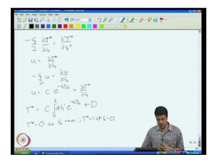
So my equation is minus psi by 2 d d T star by d psi is equal to T square T star by d psi square. So, I can solve this. Now in case so if I define u is equal to d T star by d psi then I will get minus psi by 2 u is equal to d u by d psi and u is equal to a constant e power minus psi square by four and this is equal to d T by d psi. Therefore, T is equal to c integral 0 to psi d psi prime e power minus psi prime square by four plus some other constant d.
