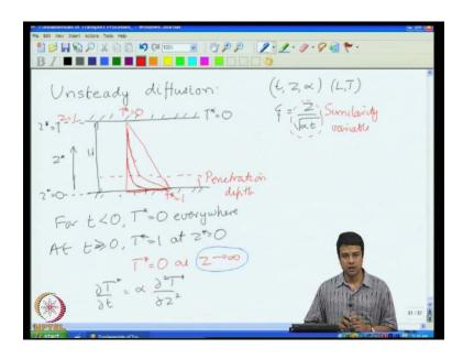
So let us go ahead with analyzing that problem. So, back to our problem two plates and I will just work in scaled coordinate Z star is this axis. I can scale by the thickness whatever the thickness is, I can scale it by the thickness to get this boundary at Z star is equal to 0 and this boundary at Z star equals 1. So, the scale distance varies between 0 and 1.
