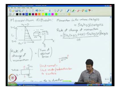
The form of the equation for momentum diffusion was slightly different. It came out of Newton's law third law, Newton's laws of motion rate of change of momentum. In a differential volume is equal to the some of the applied forces and there I had defined for you in some detail what is the stress tau x z?
