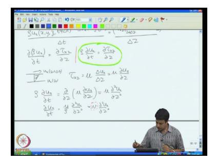
It is the force per unit area in the x direction acting at the surface with outward note outward. You are at normal in the Z direction and I also told you that if the outward unit normal is in the minus Z direction the force will be minus tau x Z because if you interchange if you if you reverse the direction of the unit normal the direction of the force also changes according to Newton's third law.
