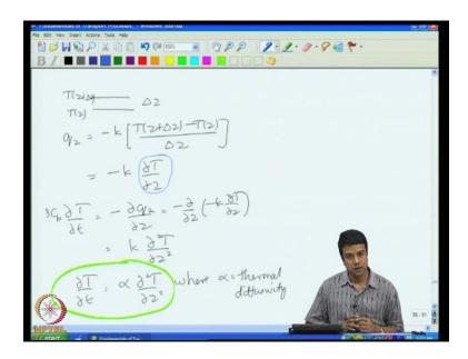
And then we need an equation for the flux. Fourier's law of heat condition q Z is equal to minus k partial T by partial Z. Note the partials here. These are important. It implies that you're taking the variation in temperature with Z keeping all other coordinates the same. That is you are varying Z a little bit and finding out the difference in temperature keeping x y and T z constant. And from that we got this diffusion equation for the temperature where alpha is the thermal diffusivity.
