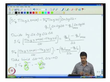
And we got a balance equation which was basically of this form rho c p into d T by d T is equal to minus partial q Z by partial z. So this basically tells you that the rate of change of specific energy within that volume is equal to the rate at which energy comes in minus the rate at which it is going out. The difference in fluxes across the two surfaces the bounding surfaces.
