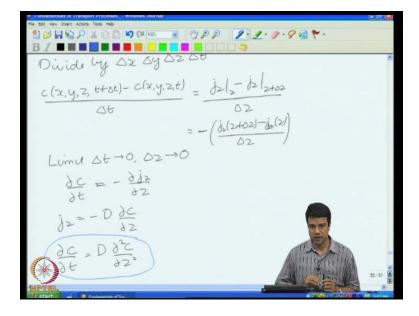
The exact same equation except that concentration is substituted for temperature; mass diffusion coefficient is substituted for the thermal diffusion coefficient. In all of these we assume that the diffusion coefficients both from mass and the thermal diffusion coefficients are not functions of position. If they are functions of position it gets a little
