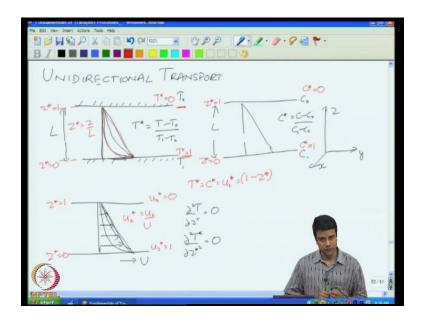
And in what is called a Cartesian coordinate system. The three coordinates are x y and z and unidirectional transport in a Cartesian coordinate system means that it, the transport is taking place only along one direction and the simplest example in Cartesian coordinates is the transport between two flat plates and we looked at various instances of heat and mass transfer between two flat plates both at steady state and at unsteady state.
