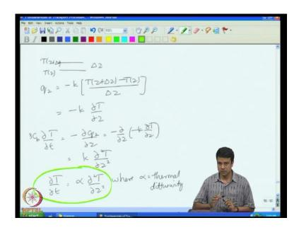
So these, all three equations which I got here, this equation for example, is the first order differential. In time differential equation, in time second order differential equation, in z you need two boundary conditions on z. For example, in the problem that we took, the two boundary conditions are at the two plates, z is equal to 0 and z is equal to L. But, it needs two boundary conditions in z and since it is first order in time you also need an initial condition.
