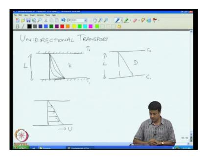
The simplest situation that one can consider is the example of the transfer between two flat plates. I have two flat plates, separated by a distance L. In the heat transfer problem, I will have a fluid of thermal conductivity k between the two plates and I will keep the temperatures of the two plates at two different temperatures, that is, T naught and T 1. Then I want to know, what is the temperature in-between the two plates?
