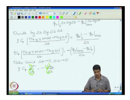
Once you do division, what you will get is that row C p into T at x y z t plus delta t minus T at x, y, z, t, the whole thing divided by delta t is equal to q z at the location z minus q z at z plus delta z by delta z. I can now rewrite this equation a little bit, on the right hand side, I can write this as minus of q z at z plus delta z minus q z at z divided by delta z.
