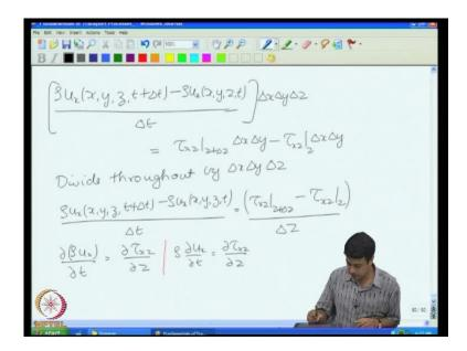
The rate of change of momentum - row u x at x, y, z, t plus delta t minus row u x at x, y, z, t divided by delta t into the volume delta x delta y delta z. This thing has got to be equal to tau x z at z plus delta z times at delta x delta y. Force on the top surface; on the bottom surface, the unit normal is in the minus z direction. The bottom surface the unit normal is in the minus z direction, so this is the balance equation.
