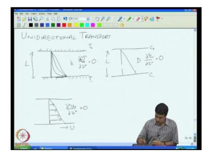
At steady state, the time derivatives are all 0. At steady state, the equations here will become d square t by d z square is equal to 0 d square c by d z square is equal to 0 and d square u x by d z square is equal to 0. So, you can solve any of the equations equivalently in order to get the steady state profiles. However, we will use one thing that will be useful later on when we do other kinds of transfer problems. However, solving these equations directly, we will scale them.
