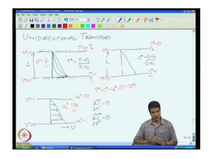
Once expressed, in this form, all 3 equations have identical forms. One could work with the form of the differential equation that is of the form d c by d t is equal to some diffusivity than d square c by d z square, and one has to solve that problems subject to the conditions on the 2 surfaces, as well as the conditions at the initial time.
