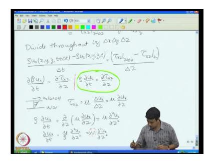
Basically, Newton's law of viscosity states that if I have two plates moving with velocity u x at z plus delta z and u x z. So, there is a linear variation in velocity between these two plates and the shear stress tau x z is equal to the viscosity times delta u x by delta z, the change in velocity divided by the separation of the 2 locations. Take the limit as delta z goes to 0, you will get this as mu times d u x by d z.
