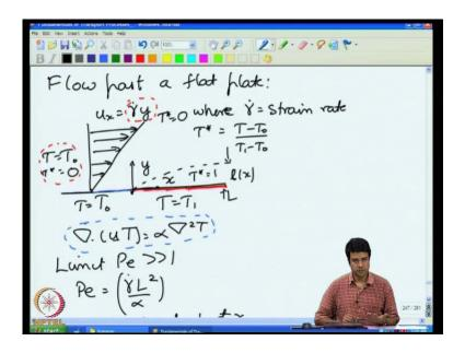
A flat plat with a heated section starting at x is equal to 0, T is equal to T naught for x less than 0 and T is equal to T1 for x greater than 0; the fluid that is incident on that plate has a temperature T naught, and we assume a linear velocity profile at the surface, the velocity u x is non zero, its equal to the strain rate times y, whereas u y is equal to 0.
