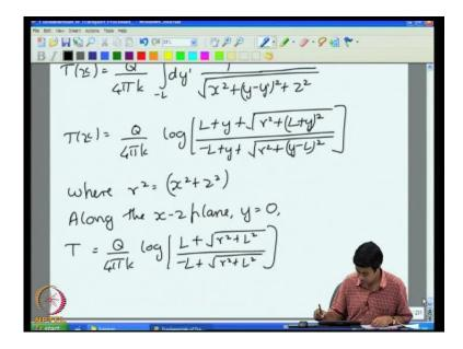
So, this of course gives us the analytical solution the question is what physically does this mean. So, as usual let us take 2 limiting cases. To simplify the problem, I will assume for the moment that we are along the x z plane y is equal to 0. Therefore, T is equal to Q by 4 pi k, log of L plus root of r square plus L square...(Refer Slide time: 45:09)
