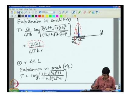
So, I have my wire along the y coordinate along the x z plane. So, I am taking the distance an observation point. That is somewhere, along this x z plane and for this observation point. The distance from the origin is the radius r and of course the solution is symmetry with respect to r. It depends upon only the distance from the axis. So, this is the solution along the x z plane.
