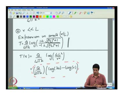
And if I expand out this log function in small r by L. Then, I will get the temperature Q by 4 pi k log of 4L square by r square. Just expanding out this function in small r by L and I can further write this as Q by 2 pi k into log of 2L minus log of r.
