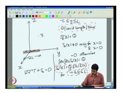
The r in this solution is the radial coordinate in the cylindrical coordinate system. In which the axis is the y axis. It comes out naturally in this form. The reason is because if I go back to the original problem. This problem: there is a wire in the y direction along the y axis. Therefore, as you go around the y axis in the x z plane. There is no change. Therefore, it will be more convenient to analyze this in a cylindrical coordinate system.
