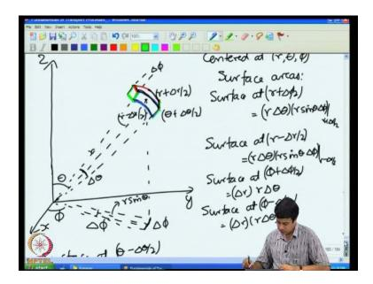
So, I have location here at which I want to construct a differential volume for carrying out my balance equations. So, this total distance is r. Now, my differential volume is centred at the location r theta and phi. That means, that that means, that it has to be bounded by surfaces at r minus delta r by 2 and r plus delta r by 2 theta minus delta theta by 2 and theta plus delta theta by 2 and phi minus delta phi by 2 and phi plus delta phi by 2.
