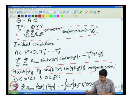
So, this initial condition is determined using orthogonality relations that I have shown you over here. You have to multiply simultaneously by the Eigen functions in both the x and the y directions and integrate to get the coefficients.
