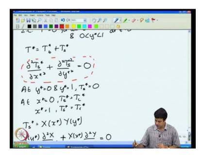
This is solved by separation of variables. Y is the homogeneous direction the boundary conditions are homogeneous in the y direction. X is the inhomogeneous direction. Therefore, the solution will be of the form of sine functions which are the basis functions for the second order derivative operator in the y direction.
