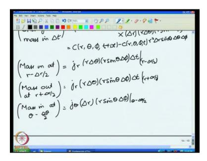
J theta times the surface area. The surface area for that surface on top is equal to delta r times r sine theta delta phi at theta minus delta theta by 2.
