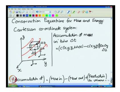
So, when we looked at transfer in a Cartesian coordinate system in the last class I had defined for you a differential volume which was in the form of a cube.
