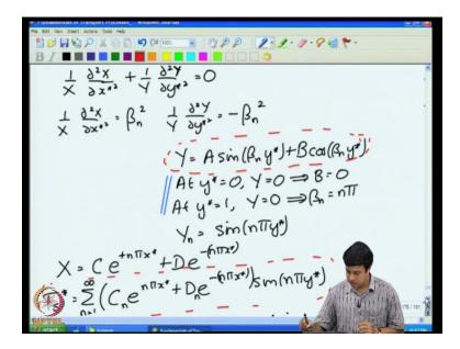
So, in the y direction because the boundary conditions are homogeneous I will get sine and cos functions where the Eigen values beta n are determined from the condition that Y has to be 0 on both surfaces. If Y is homogeneous then x is inhomogeneous you get sine exponentially increasing and decreasing solutions in the x direction.
