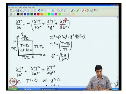
And then we had solved an equation for the conduction in a cube in the previous class; the unsteady heat conduction and I showed you how to do the separation of variables for that particular case. So, when one does separation of variables in three or more variables.
