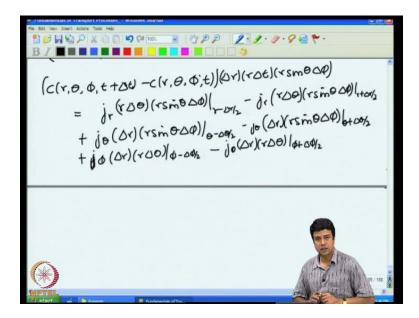
So, this gives me the concentration first, C at r theta phi t plus delta t minus C at r theta phi t into the volume. This is going to be equal to the sum of all the mass in and out due to fluxes.
