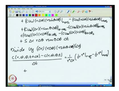
So, I will have convection terms C u r times r delta theta into r sine theta delta phi at r (no audio 48:39 to 49:40)). So, those the terms due to convection and finally, I am going to get a source term plus s delta r r delta theta r sine theta delta phi and delta t. So, those are there is the final expression for the difference equation and in order to get the differential equation as usual I divide by delta t and I divide by volume.
