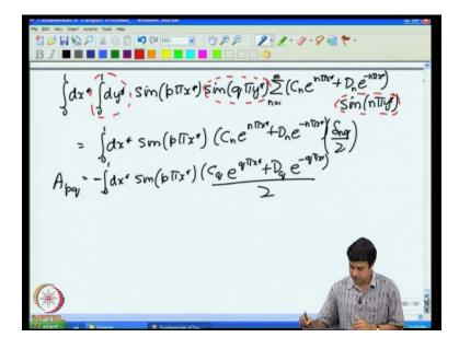
And that gives us the final solution for the coefficients. We have the solution for the transient problem, we have the solution for the steady problem. Put those together and you will get the total temperature field. So, that is how you extend separation of variables to this particular case. As I told you in the previous lecture, we are now going to go and
