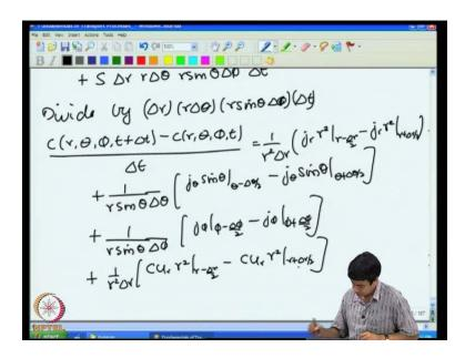
So, that will give me 1 by 1 by r sine theta delta theta into j theta times sine theta at theta minus delta theta by 2 minus j theta times sine theta at theta plus delta theta by 2. So, that was for the variation in the theta direction because the surface area is changing.
