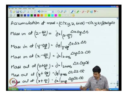
And then, we had written the mass conservation equation; accumulation of mass is equal to mass n minus mass out plus production in the volume and the differential volume is chosen with a certain logic.
