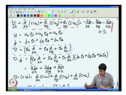
So, we saw this general equation for conservation in three-dimensions here. And I showed you how to write that in a more compact form. We defined the vector velocity, velocity is of course a vector, it has three components. The vector flux, once again this has three components. Flux gives you a rate of transport in one particular direction perpendicular to a surface, so it has a direction associated with it.
