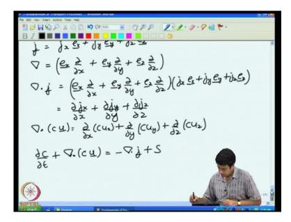
So, if I use these then the equation gets considerably simplified. The equation is just dc by d t plus del dot C times u. Note that this operator is acting on both C and u is equal to minus del dot j plus any sources that are present. So, for a three-dimensional system this
