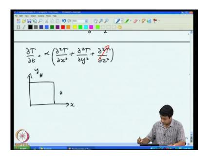
So, this is an unsteady state diffusion problem. So, let us start, no velocity therefore the equations are dT by dt is equal to alpha times d square T by dx squares plus... There are no sources or sinks within this volume.
