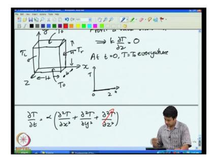
Note that the front and back faces are insulated; that means, that k times dT dz is equal to 0 on the front and back faces. That means, if I plot the temperature as a function of Z along the cube from 0 to H, the slope is 0 here, the slop is 0 here.
