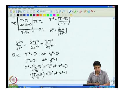
On the left face T is equal to T l therefore, T star is equal to T l minus T naught divided by T naught. And I will call this as T l star at x star is equal to 0 and is equal to T r minus T naught by T naught is equal to T r star at x star is equal to 1. So, those are the boundary conditions on the bottom, top, left and right.
