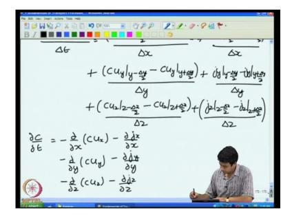
So, therefore, this term is partial is negative of d by dx of C u x, because the derivative is the values at x plus delta x by 2 minus the value at x minus delta x by 2 divided by delta x. So, this is the negative of that derivative. Minus partial j x by partial x minus d by dy of C u y minus partial j y by partial y minus d by d z of C u z minus partial j z by partial z. I can put this equation in a more compact form.
