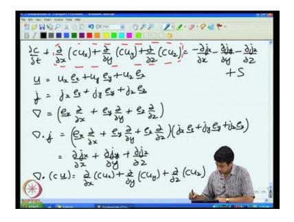
I should have the source term S over here. So therefore, I can write the right hand side as minus del dot j, where del is a vector, j is a vector. Similarly, this three terms on the left hand side I can write as del dot C u vector, which will be equal to d by dx of C u x plus d by dy.
