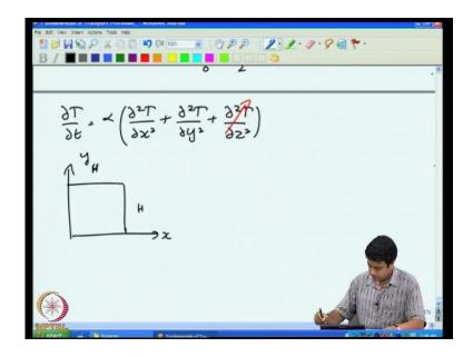
So, therefore, the variation of temperature with z becomes identically equal to 0 and one can neglect variations in the z direction. So, in that case it becomes a two-dimensional problem. Two-dimensional problem, x y on a square of side H, where I have on the top and bottom faces, I have T is equal to T naught and T is equal to T naught, T is equal to T l on the left phase and on the right phase T is equal to T r, the temperature on the right face.
