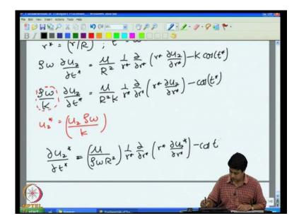
So, I should define u z star is equal to u z rho omega by k I should be defining u z star in this manner and if I define u z star in this manner my equation will become d u z star by d t star is equal to mu by rho omega R square 1 by r d by d r of r d u z star by d r minus cos t and this of course, this is 1 over the Reynolds number, this is the inverse of the Reynolds number 1 divided by the Reynolds number.
