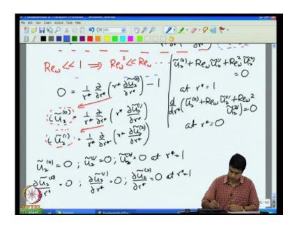
So, now each of these equation individually has to be equal to 0; it was that implies is that 0 equal to 1 by r d by d r of r d u z by d r minus 1. So, that is the order one equation. The first correction is i u z 1 I am sorry i u z naught is equal to 1 by r d by d r of r d u z 1
