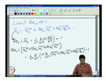
So, we will come back to this little later, what happens in the limit Re omega small compared to 1, I can consider the Reynolds number as a small parameter in that case, I can expand my velocity; I can expand u z tilde is equal to plus plus etcetera. So, I am using an expansion for the velocity field in this small parameters, the original equation that I had was i u z tilde is equal to minus 1, so that was the original equation that I had.
