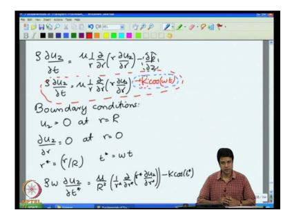
So, we have a differential equation for the velocity field, which contained an in homogenous term, this equation for the velocity field contain in a homogeneous term that was k cos omega t. The boundary conditions for the the flow through the pipe, no slip conditions at the wall, the velocity has to be equal to 0 at the wall, at r is equal to capital R; at r is equal to 0 we have the symmetric condition, that we had discussed earlier.
