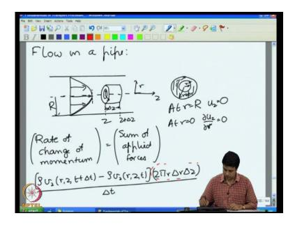
And then, we had started looking at the flow in a pipe and doubtless needless to say this is commercially important flow. And the way we solve this problem was to first consider a cylindrical shell and apply the momentum balance condition; rate of change of momentum is equal to sum of applied forces on the surfaces.
