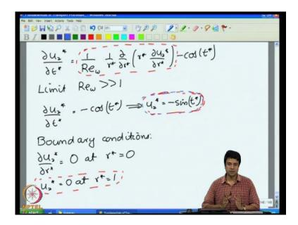
So, therefore, the equation can be written as d u z star by d t star is equal to 1 over Re omega minus cos of t. So, as I said I am considering the limit of high Reynolds number I
