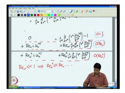
So, if Re omega where identically equal to 0 then, I could neglect all the terms proportional to Re omega and I would get on on the left hand side, I will just get 0 because, in the left hand side I have Re omega is multiplying by everything. So, on the left hand side I will just get is 0, on the right hand side I will get is equal to minus 1. So, these are term are independent of Re omega in the limit as Re omega is goes to 0.
