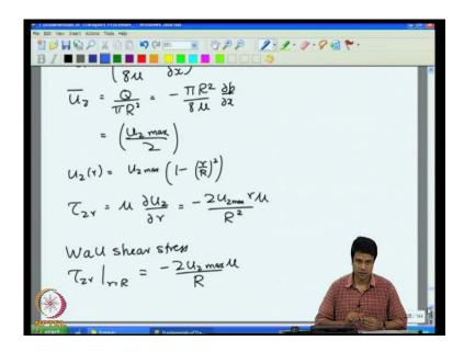
From that, we got shears stress, the shears stress at any point in the fluid and the shears stress at the wall by setting r is equal to capital R and from this, we got the shears stress as the function of the maximum velocity, we know how the maximum velocity is related to the pressure gradient. So, you get the shears stress as the function of pressure gradient.
