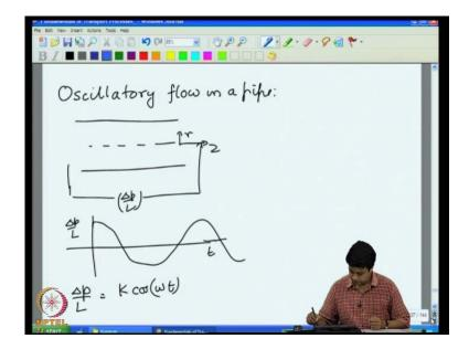
In this particular case, we took that oscillatory function to be cos of omega times t, where omega is the frequency of oscillation; however, this procedure can be used for any type of time periodic flows, because any periodic function can be expressed as the sum of sine wave of or cosine wave of that frequency plus it's higher harmonics.
