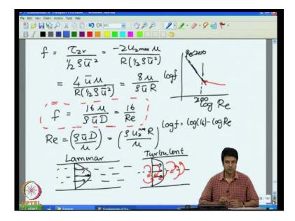
And from that, we got familiar friction factor verses Reynolds number relationship, f is equal to 16 by Re the for the laminar flow in a pipe and as I told you in the last class, the laminar flow is valid, when the Reynolds number is less than about 21 100, when the
