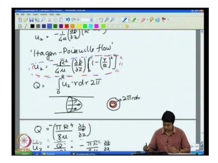
And, we had solved this to obtain the Hagen Poiseuille law for the flow in a pipe as the function of the pressure gradient. And of course, this gives you the variation velocity along the radial direction, the total volumetric flow rate through the pipe, if its volumetric flow rate I should not be having a density there.
