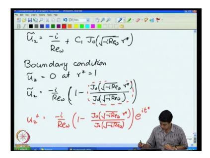
So, therefore, u z is equal to minus i by R e omega plus C 1 j naught of square root of and C 1 is of course, evaluated from the constant from the Boundary condition that we have no yet used that is the there is the Boundary condition u z tilde is equal to 0 at r star is equal to 1 and using that condition we can easily get the velocity profile as...
