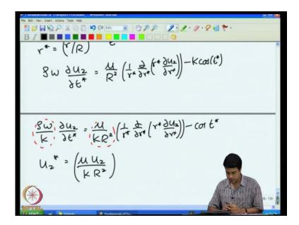
If I just write down the scaling for the time and special coordinates I will get an equation of the form rho omega du z by d t star is equal to mu by r square minus K cos t star. So, that is the equation that I get in terms of the scaled coordinates.
