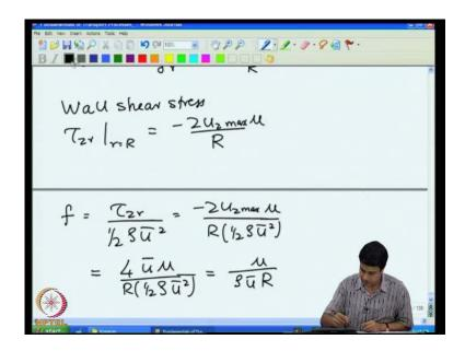
Wall shear stress tau z r at r is equal to R at the wall of the pipe is equal to minus two u z max by R, and as we had discussed in the beginning when we did dimensionless numbers the friction factor f is defined as the wall shear stress by half rho u bar square.
