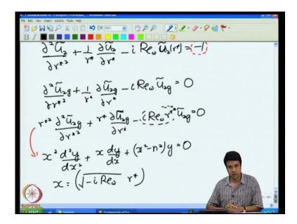
So, now, I can simplify this equation. I will get 1 by d square u z by dr star square plus 1 over r du z by dr minus i R e omega u z is equal to minus 1. So, I have taken minus this plus 1 to the left hand side and I have taken the r e dependence on the right hand side. So, this is the differential equation that I have to solve in order to get what is u z.
