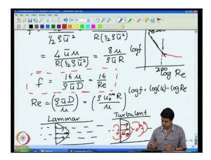
So, I finally, get 16 mu by rho u bar times D, where D is the pipe diameter this is 16 by R e, where R e is the Reynolds number rho u bar t by mu based upon the average velocity and the diameter of the pipe, this also is equivalent to rho times u z max r by mu because r is equal to d by two and u z max is equal to two times u bar.
