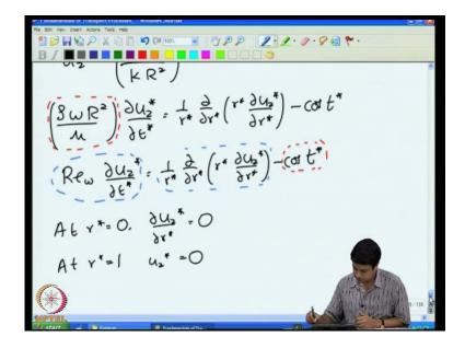
So, if I insert this into the equation ,I am getting rho omega r square by mu du z star by dt star is equal to 1 by r d by dr of r d u z star minus cos t star. And this is basically a Reynolds number based upon the frequency of oscillations and the tube radius. So, this I can define it as some number R e omega minus cos of t star.
