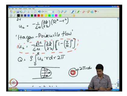
So, I had solved this equation subject to boundary conditions to get a parabolic velocity profile; u z is equal to minus 1 over four mu t p by dz into R square minus r square. Now, we had calculated the total volumetric flow rate of fluid. The volumetric flow rate is equal to the velocity times the cross sectional area. The volumetric flow rate is equal to the velocity u z times the cross sectional area along the cross section of the cylinder. Of course, the velocity depends upon r.
