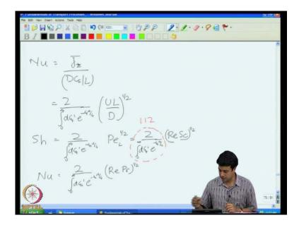
And this was once again based on similarity solution. But, not on dimensional analysis we just used the fact that the equations for the unsteady flow and for this situation are exactly the same, boundary conditions are the same. So, the solution is the same. That works for any linear problem if the if the problem is linear in the concentration field and you have well specified boundary conditions there exists solution and that solution is unique.
