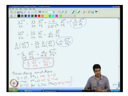
So, we had converted the equation from independent variable z and T to the independent similarity variable psi. And sure enough we ended up with an equation which was an
