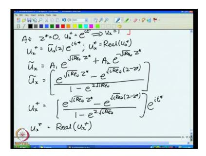
So, from this I will get u x plus which is equal to into e power i T star and then u x star will be equal to the real part of u x plus. So, that will be my final solution. Of course, I could evaluate this real part numerically and then find out the velocity profile at very point within the flow.
