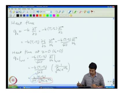
And the similarity solution basically reduces the partial differential equation to an ordinary differential equation on the basis of dimensional analysis. You can calculate the flux and the flux decreases at T power minus half as time progresses.
