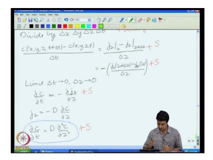
In the case of mass transfer we get an equation that looks exactly the same except that the concentration is substituted for the temperature and the mass diffusion coefficient is substituted for the thermal diffusion coefficient.
