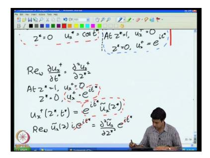
So, my equation is R e omega d u x plus by d T is equal to d square u x plus by d T and T d z square with boundary conditions at z star is equal to 1 u x plus is equal to 0 and at z
