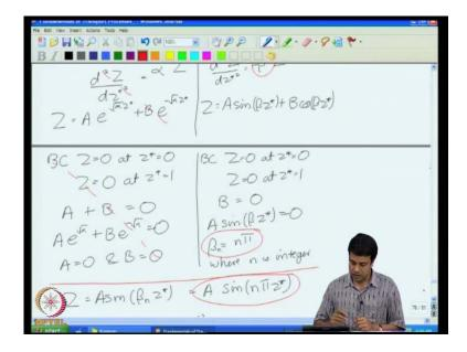
If my solution which is of form sine and pi z pi z star then this is 0 both at z is equal to 0 as well as z is equal to 1 provided n is an integer. So, the boundary conditions place a restriction on this constant beta. The boundary conditions place a restriction on the constant beta not just on the constants you get from the solving the differential equations a and b. So, these are the Eigen values for this problem.
