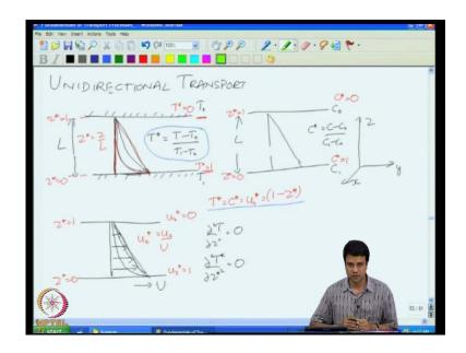
So, for example, the transport between two flat plates in the case of heat transfer problem there are two plates kept at two different temperatures T 1 and T 2 and there is transport of heat between these two. The case of concentration two plates at two different concentrations of solute c 1 and c 2 and then there is transport between these two due to the difference in concentration. The fluxes in the case of heat transfer are given by
