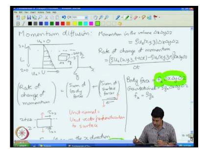
In the case of momentum transport; the route that we followed to get the momentum transport equation was a little different from heat and mass transport. In the case of momentum transport the fundamental equation that we used was that the rate of change
