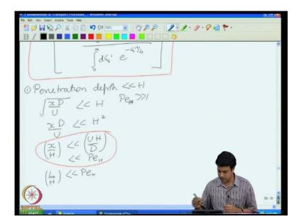
When we derive these equations the first assumption was that the penetration depth is small compared to the height H and that is when one by H the length of the film divided by the thickness is small compared to a peclet number based upon H.
