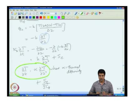
And an all these three cases we get remarkably similar equations for heat mass and momentum. So, for example, in the case of heat transfer we get an equation of this form; the time variations of temperature is equal to the diffusivity times the second derivative with respect to the z coordinate. The z coordinate is the coordinate in which there is variation of temperature plus any source of heat that is there.
