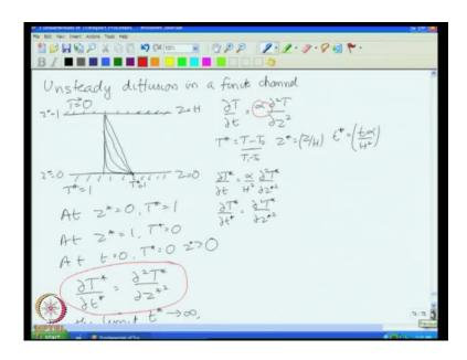
So, the problem that we were considering was as follows: This was unsteady diffusion in a finite channel; I have 2 plates, 0 and H, the temperature at the bottom is one, the temperature of the top is 0 in scaled variables.
